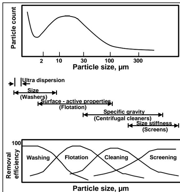
Figure 1 : Particle size distribution in a recovered paper pulp suspension and unit operation removal efficiency. Mc Cool 19871
